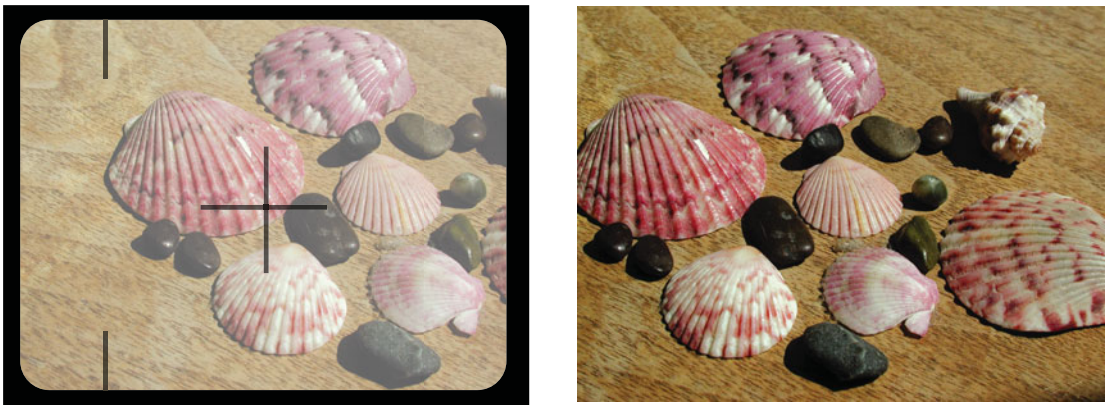
FIGURE 5.17 When you shoot at close range, what you see through the viewfinder of a rangefinder camera is not what your camera will actually shoot. Parallax guides give you an indication of where the real edges of the image are. The image on the left shows the view through the viewfinder, and the image on the right shows the resulting picture. Notice that the parallax lines allow you to correctly frame the left side of the image, even though you can't see the right side (because you're too close to the subject). If a camera's viewfinder is above the lens rather than next to it, the camera will exhibit parallax shift vertically rather than horizontally.
